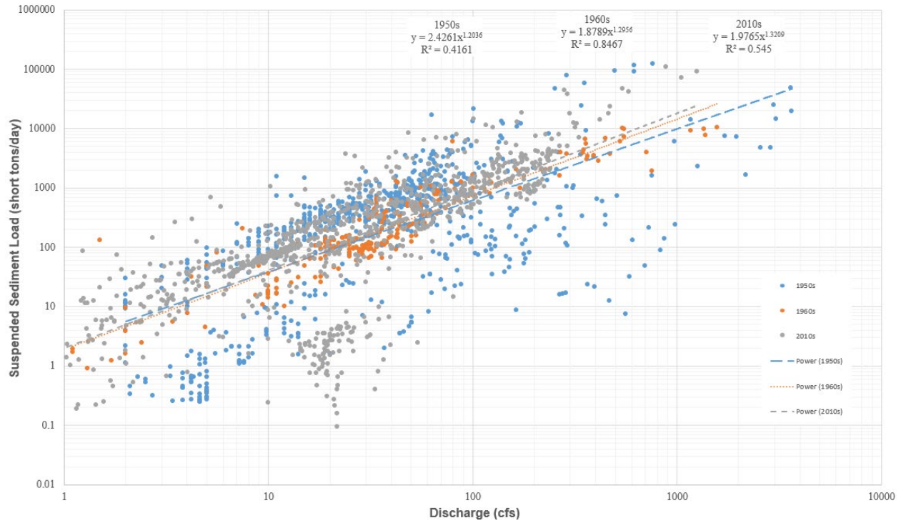
Figure 1. Suspended sediment rating curves for suspended sediment loads versus daily average discharge. Power regression equations are shown in the upper portion of the graph.
